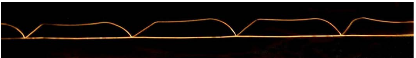
Figure 1: Heytether with one basic wire and one auxiliary tether loop
