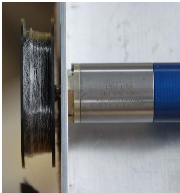
Figure 9: The upreeled tether after the second test run.
