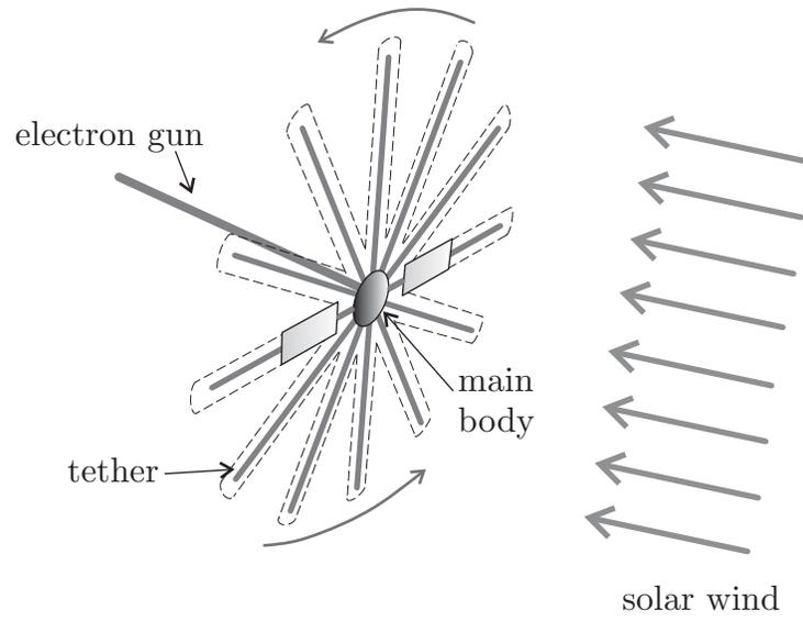
**Figure 1. Schematic view of E-sail concept.**
