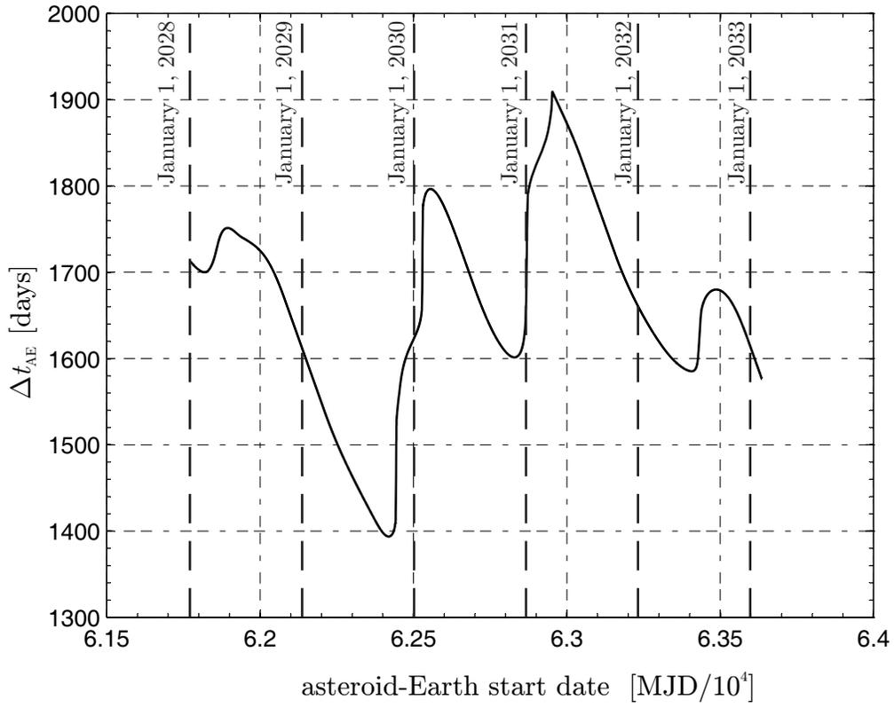
**Figure 8. Asteroid-Earth minimum transfer time as a function of the Modified Julian Date for  $a_{\oplus} = 0.1 \text{ mm/s}^2$ .**
