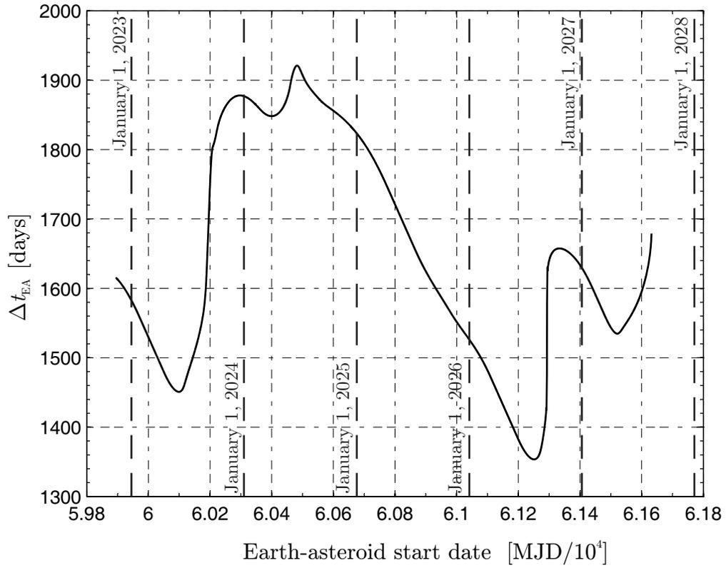
**Figure 7. Earth-asteroid minimum transfer time as a function of the Modified Julian Date for  $a_{\oplus} = 0.1 \text{ mm/s}^2$ .**
