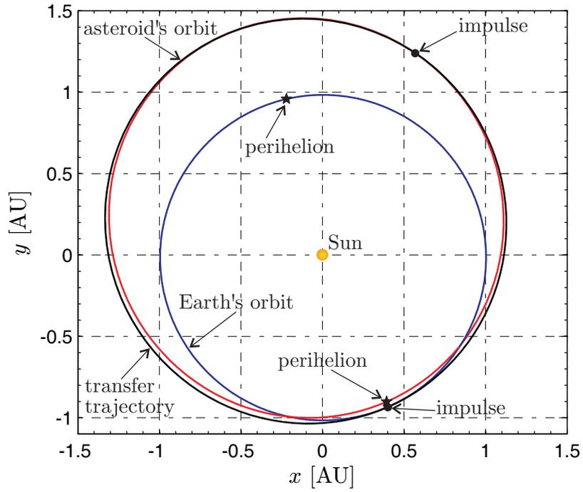
**Figure 4. Two-impulse transfer trajectory with minimum velocity variation (orbit-to-orbit transfer).**
