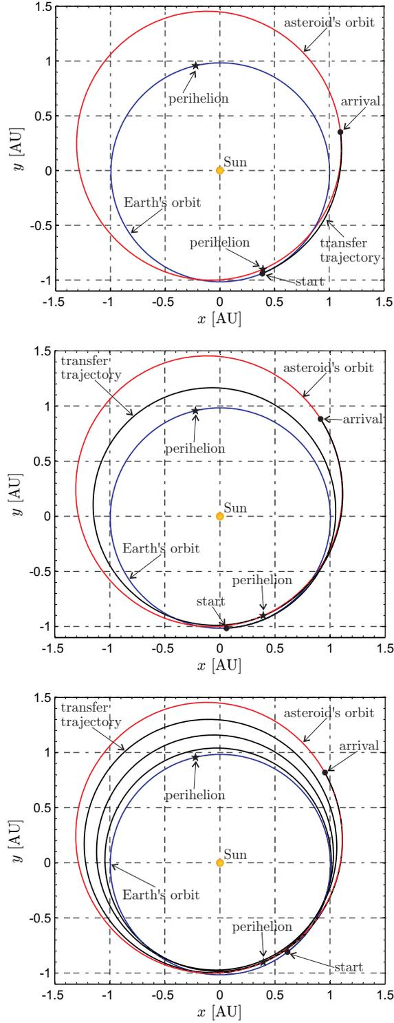
**Figure 5. Ecliptic projection of the (orbit-to-orbit) optimal Earth-asteroid transfer trajectory for  $a_{\oplus} = 1 \text{ mm/s}^2$  (top),  $a_{\oplus} = 0.2 \text{ mm/s}^2$  (middle),  $a_{\oplus} = 0.1 \text{ mm/s}^2$  (bottom).**
