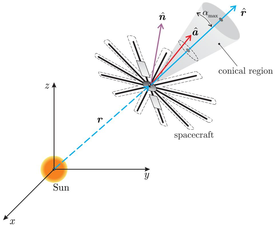
Figure 2. Spacecraft propulsive thrust vector direction.
