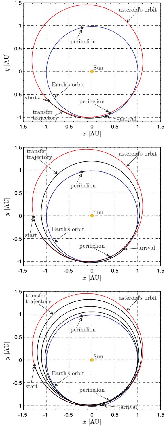
Figure 6. Ecliptic projection of the (orbit-to-orbit) optimal asteroid-Earth transfer trajectory for  $a_{\oplus} = 1 \text{ mm/s}^2$  (top),  $a_{\oplus} = 0.2 \text{ mm/s}^2$  (middle),  $a_{\oplus} = 0.1 \text{ mm/s}^2$  (bottom).
