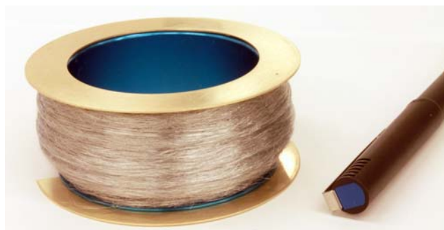
Fig. 6. Produced 1km tether on production reel (Tanaka AL-2 reel with additional side walls).
