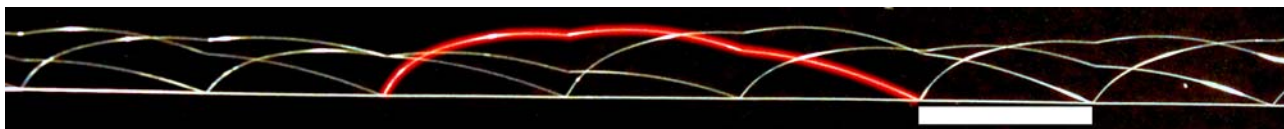
Fig. 5. 4-wire Heytether. This sample was produced right after the 1 km production. The white bar is 10 mm long. One full loop is highlighted (red).
