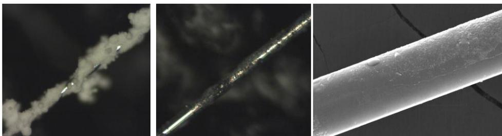
*Fig 1. Various coating methods. (left to right) hBN,  $WS_2$ , and  $H_2O$  vapor. The two sprays were applied from a distance of 20 cm for 2 sec. Water vapor was applied for varying times, 30 min pictured.*
