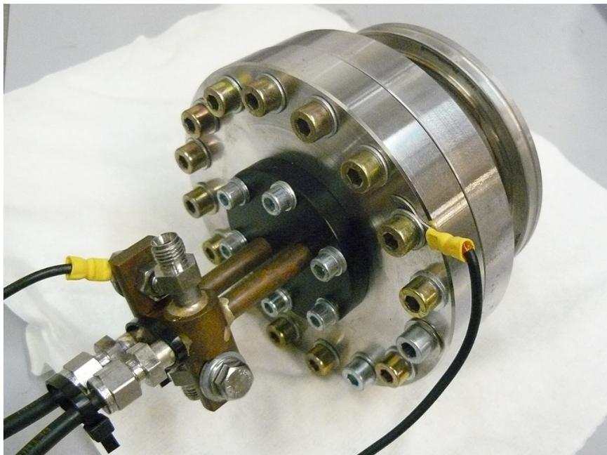
Figure 5. Filament vacuum feed-through for electron gun.
