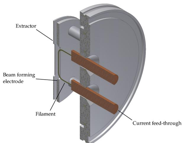
Figure 6. Preliminary design of the two-electrode slit-beam electron-gun.
