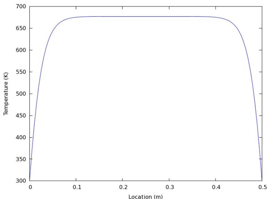
**Figure 3.** The spatial temperature distribution of the wire with 25 mA heating current.
