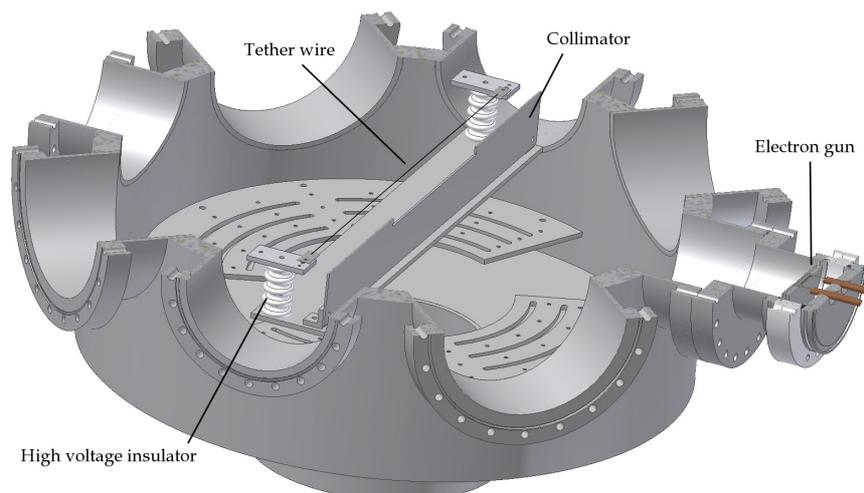
**Figure 7.** Section view of the vacuum chamber with equipment for emissivity measurements and electron bombarding.
