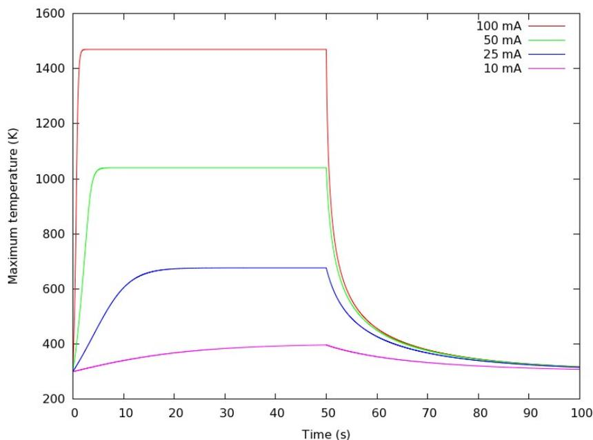
**Figure 2.** Maximum (central) temperature of the wire as a function of time with different heating currents. The heating current is switched off at t=50 s.
