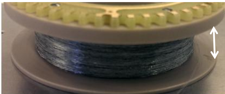
Fig 1. 100 m of 4-wire Heytether on an Aalto-1 flight reel. There are 15 layers of tether on the reel. The tether is uniformly distributed over the available space (1 cm, indicated by an arrow).
