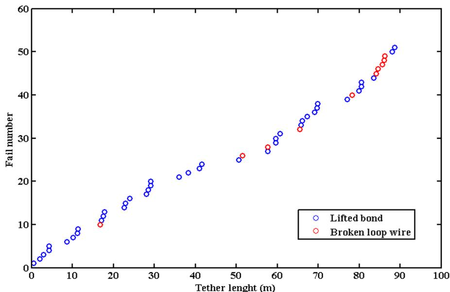
Fig 3. Bond failure analysis for the manufactured tether. The failure rate is reasonably constant during the production. However, the ‘Broken loop wire’ failure mode is more prevalent in the later stages of production.
