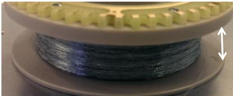
*Fig 1. 100 m of 4-wire Heytether on an Aalto-1 flight reel. There are 15 layers of tether on the reel. The tether is uniformly distributed over the available space (1 cm, indicated by the white arrow).*
