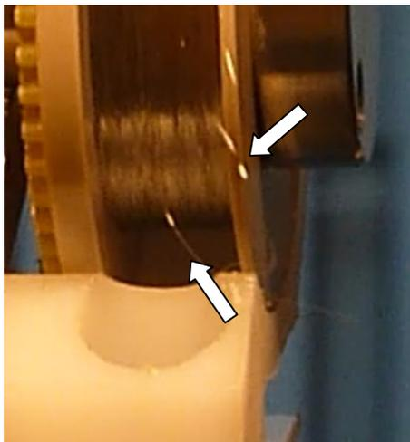
*Fig 4. A broken loop wire on the reel (lower arrow) causes the tether (upper arrow) to jam on the tether outlet.*
