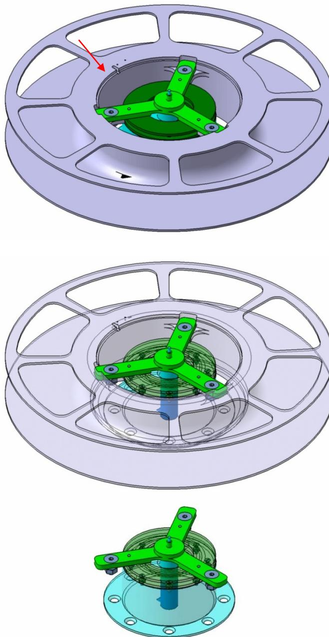
Figure 6: Reel configuration, on top the position of the tether hole is marked with an arrow, in the middle the reel (gray) and the motor holder (turquoise) are Transparent to show the position of the motor, below the ... is shown without the reel
