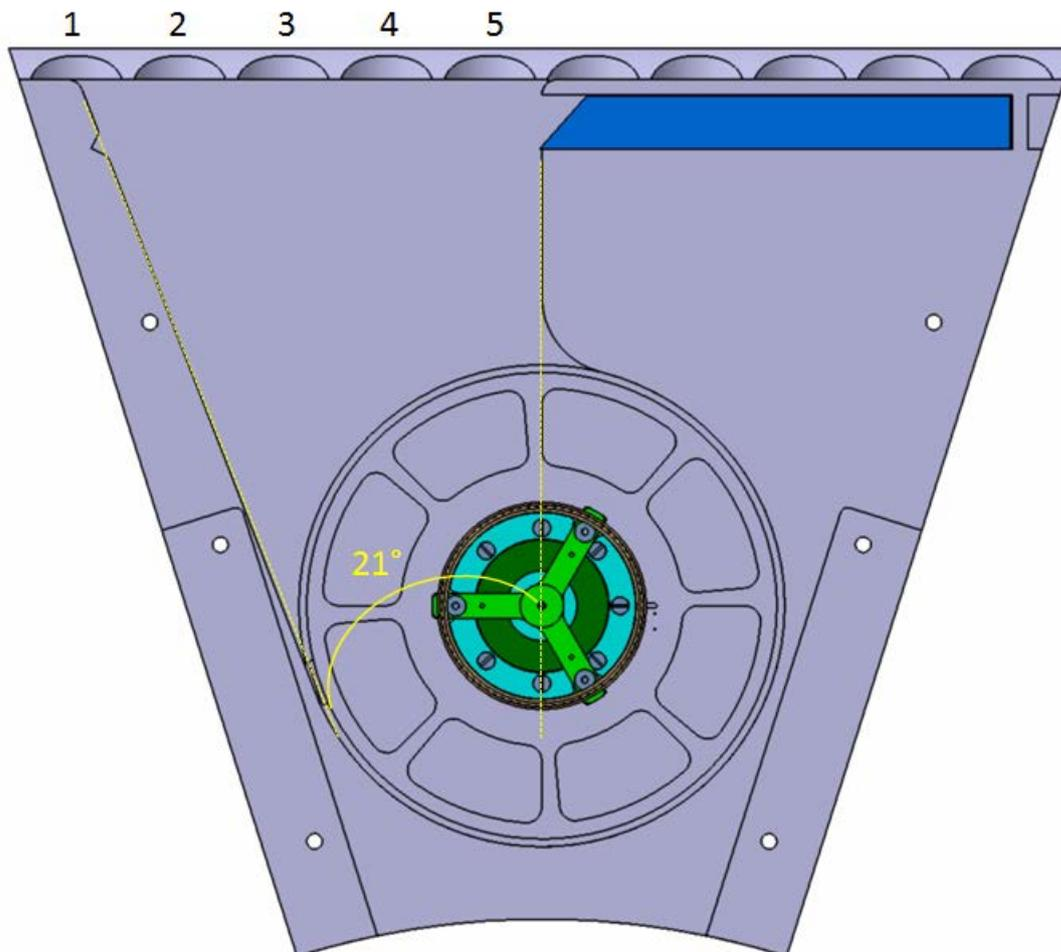
**Figure 5: Top view of the deployment mechanism**
