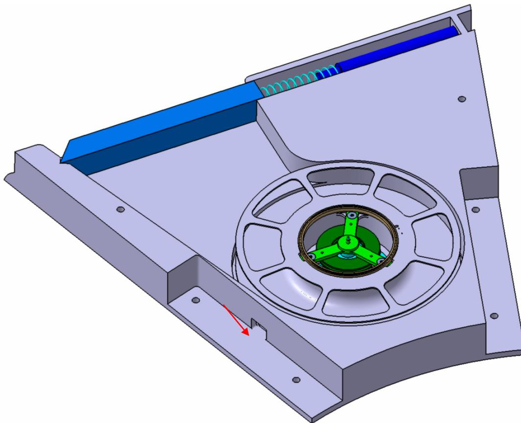
Figure 4: Deployment mechanism main reel
