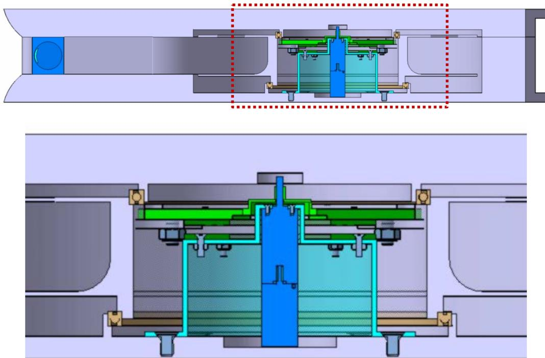
Figure 7:Section view of the reel axis: on top the whole deployment mechanism with cutter and cut out; below cut out: ball bearings (light brown), motor holder (turquoise), motor with gear box (blue), Slip ring and slip ring contactor (dark green), torque transmitter (light green), screws (dark gray), reel (gray), support structure (gray)
