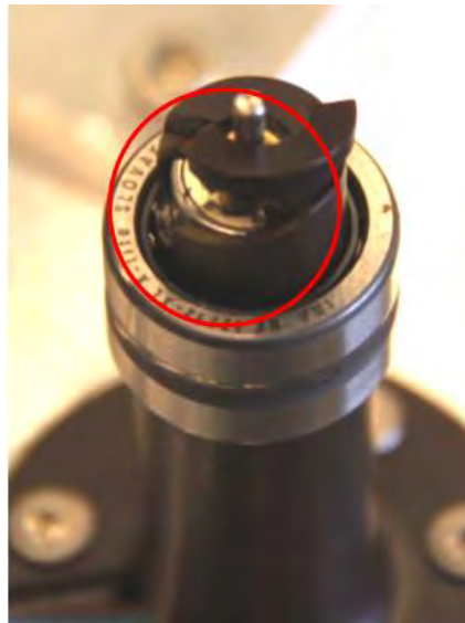
Figure 3: Damaged motor holder, the broken part is placed on top of the motor holder.
