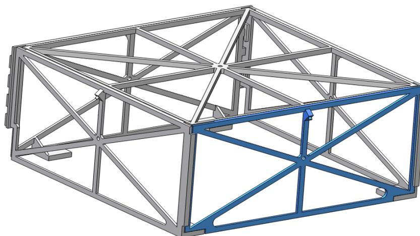
Figure 1.12: Thermal box completed with its front part (blue) put into place. (Assembling step 3.)
