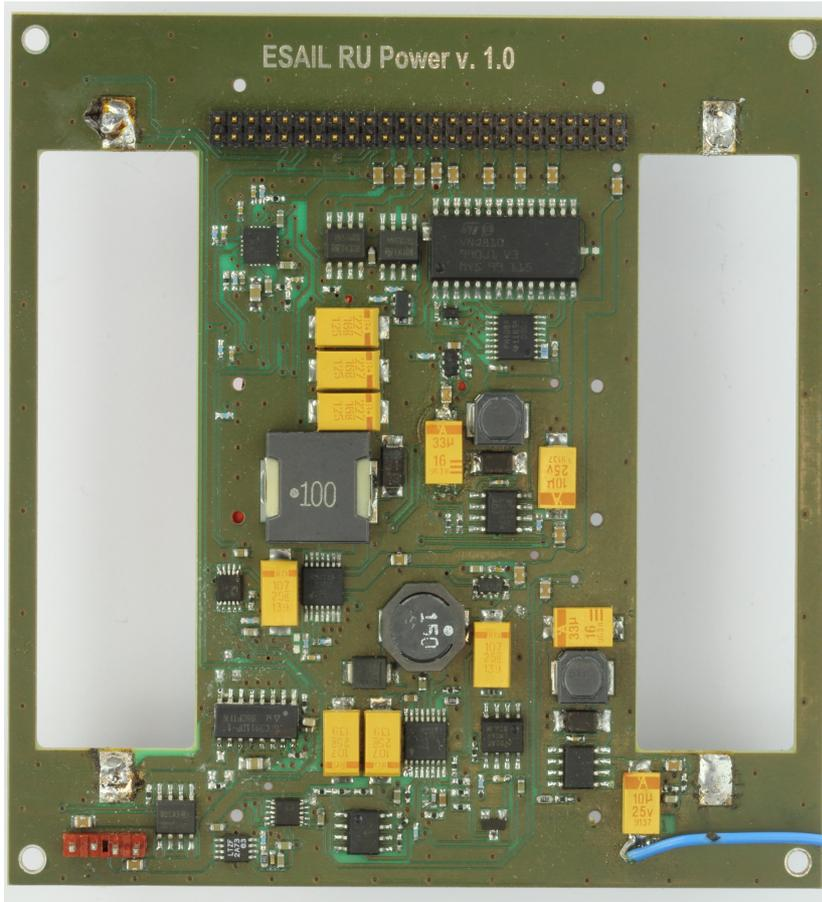
Fig. 2.1 Photo of the first prototype of the RU Power system PCB
