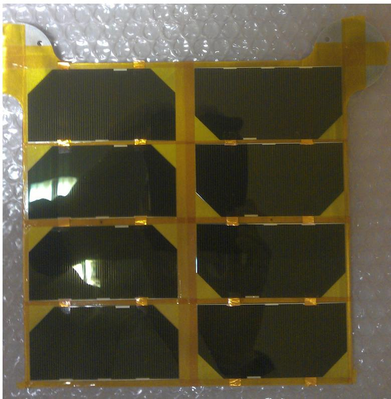
Fig. 2.5 The heatshield with polyimide tape applied and the polyimide mesh forming the recesses for solar cells (with solar cells inside, copper strips to bottom electrodes have been soldered). After this the RTV silicone was applied (the left string was rotated 180 degrees in the final design).
