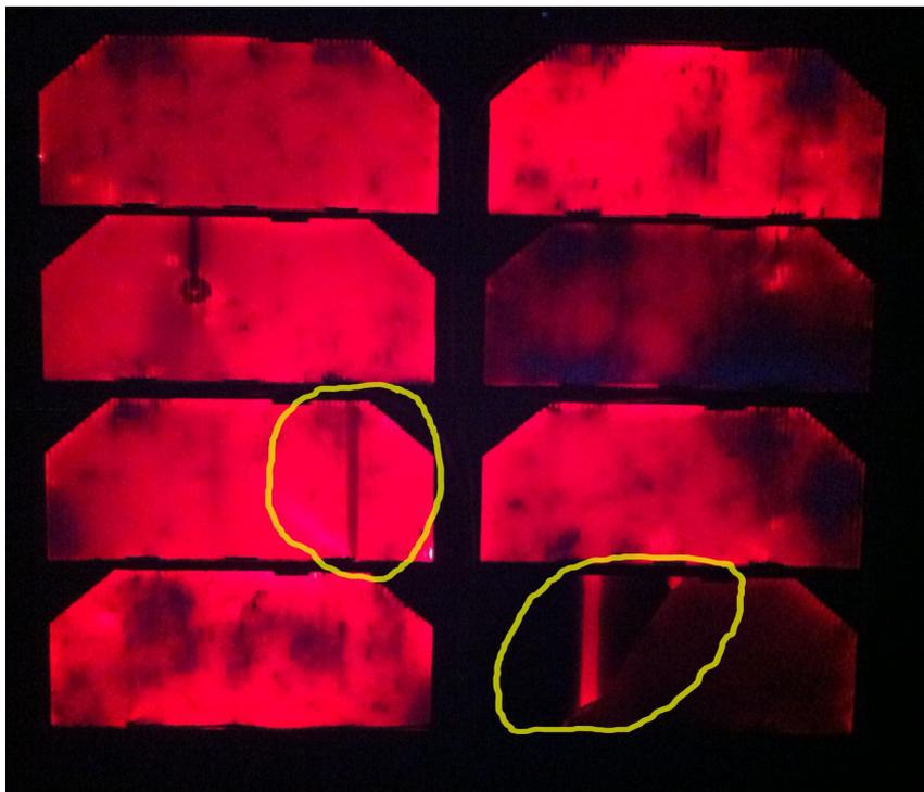
Fig. 3.2 Damaged areas of the solar cells
