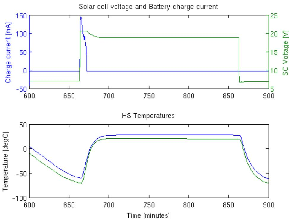
Fig. 3.1 Solar cells output and temperatures vs. time during 0.9 AU Sun simulator test.
