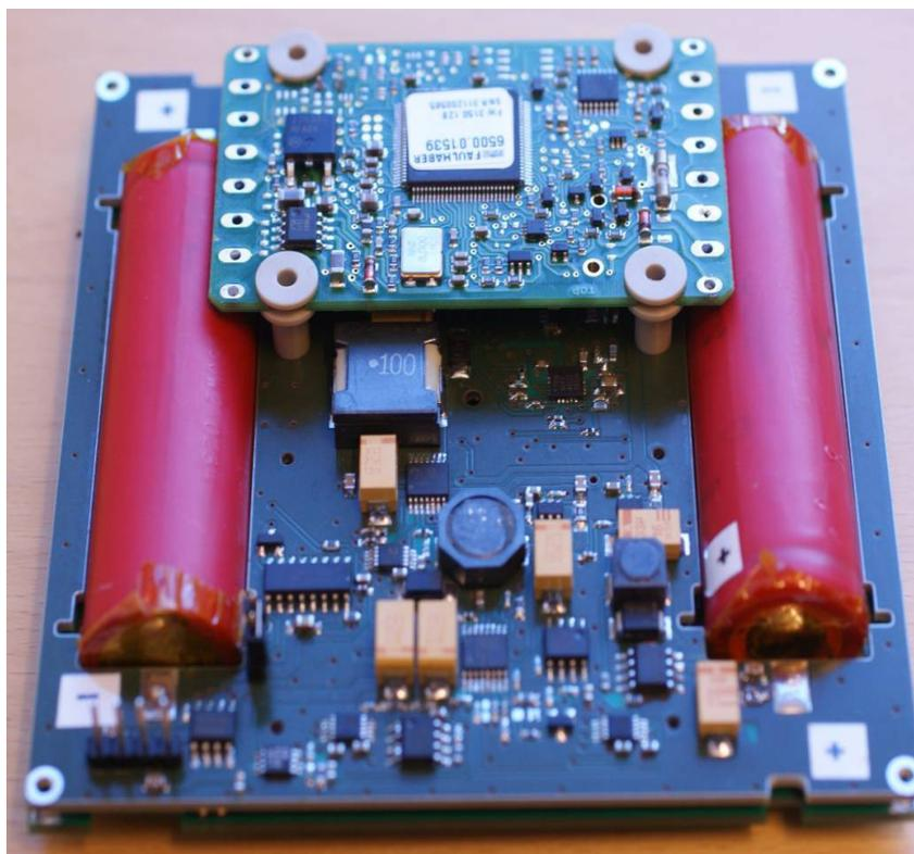
Fig. 2.4 Photo of the RU power system second prototype board
