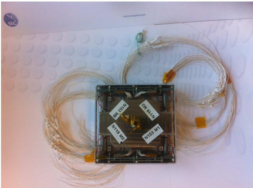
Fig. 5. NanoSpace CubeSat module with the tank in the center and four thruster modules with the thruster chips placed in the corners of the module.
