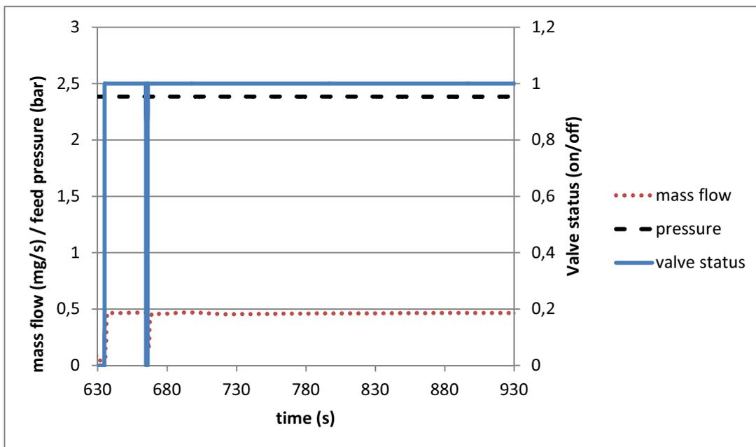
Fig. 8. Measured feed pressure, mass flow and valve status (equals zero when valve is closed and 1 when open) during a five minute interval.
