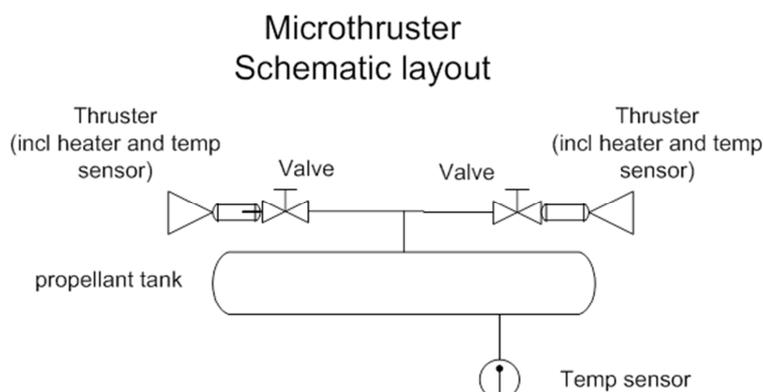
Fig. 1: Schematic of cold gas micropropulsion system.
