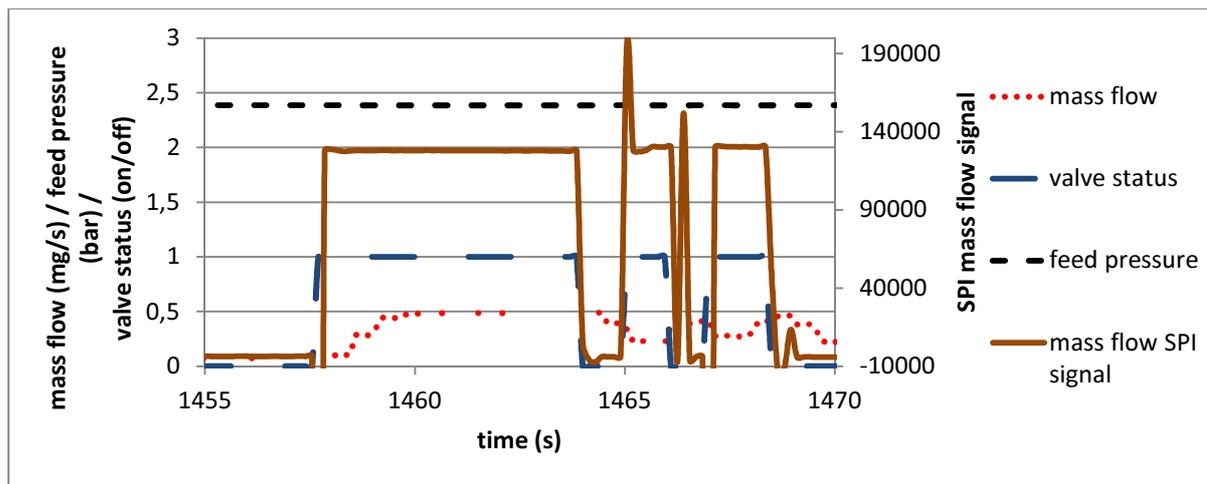
Fig. 10. Measured feed pressure, mass flow (from integrated and external sensors) and valve status during short on/off cycles of the solenoid valves.
