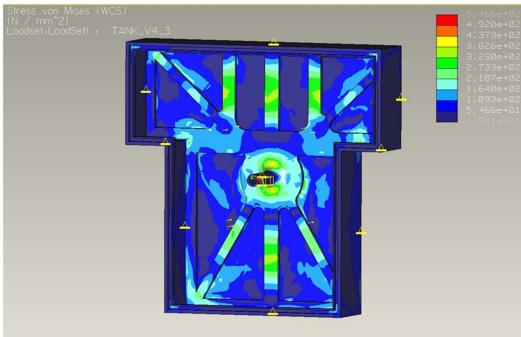
Fig. 3. Proof pressure case from the mechanical analysis.
