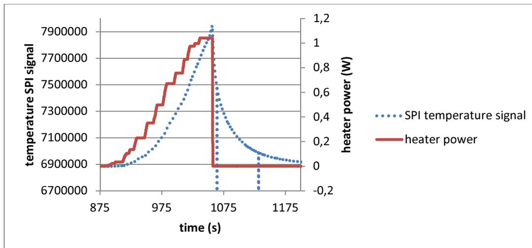
Fig. 7. On-chip integrated temperature sensor SPI signal response as the power supplied to the integrated heater is increased and switched off.
