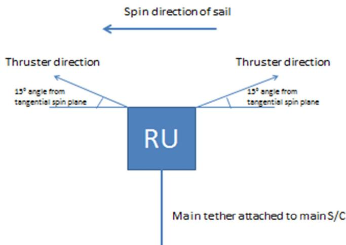
Fig. 2: Cold gas thruster positions and orientation on the RU.
