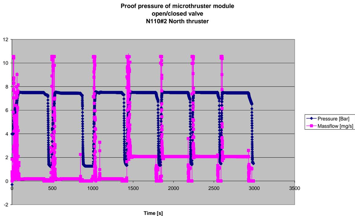
Fig. 9. Testing of solenoid valve at 7.5 bar feed pressure. The proof pressure was applied for 5 min and 3 cycles with the solenoid valve closed and then the same procedure with the solenoid valve opened.
