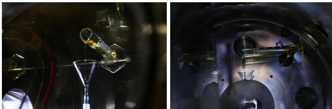
Figure 21: Propellant pouring procedure (second test campaign).
