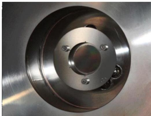
*Figure 19: Micro channel plate detector.*
