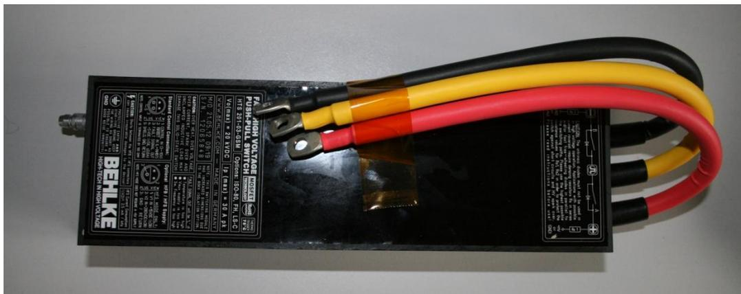
Figure 15: Fast high voltage switch used for the ToF measurements
