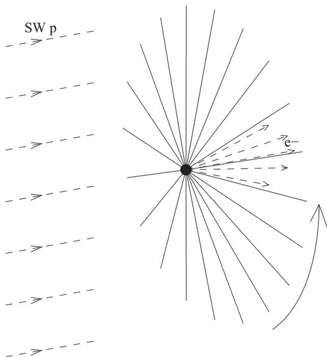
**Fig. 1.** Technically realisable version of the electric sail which consists of a set of rotating, charged tethers. Each tether forms around itself an electric influence region where solar wind proton trajectories are deflected and the tether experiences a push from the solar wind which depends on the tether's potential.
