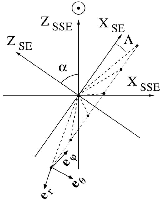
**Fig. 2 Two coordinate systems of SE (Sail Eccentric) and (Sail-centric Solar Eccentric).**
