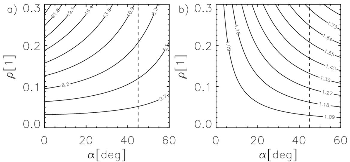
**Fig. 3 Equicontours of the coning angle (a) and the amplitude ratio of the tether rotation rate (b).**
