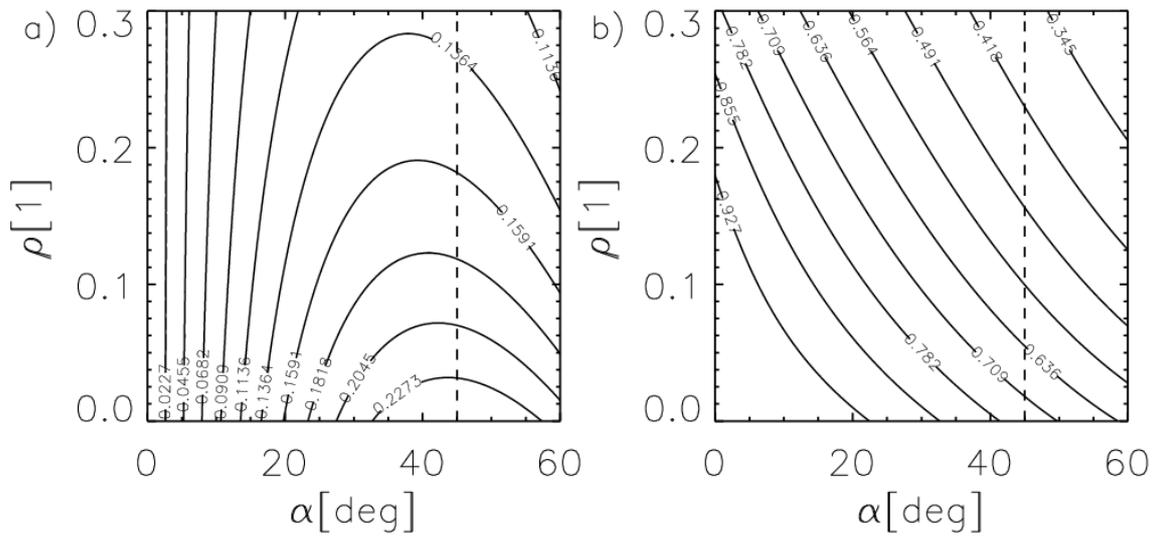
**Fig. 4 Equicontours of the total thrust in azimuthal and radial directions. The contour levels are scaled to maximum at ( $\rho = \alpha = 0$ ).**
