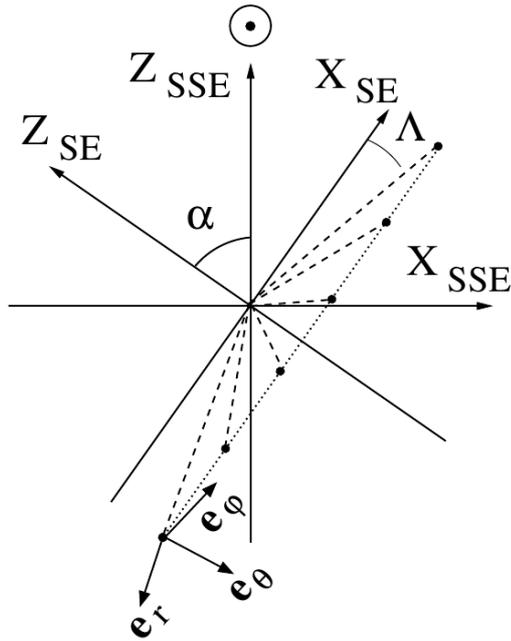
**Fig. 2 Two coordinate systems of SE (Sail Eccentric) and (Sail-centric Solar Eccentric).**
