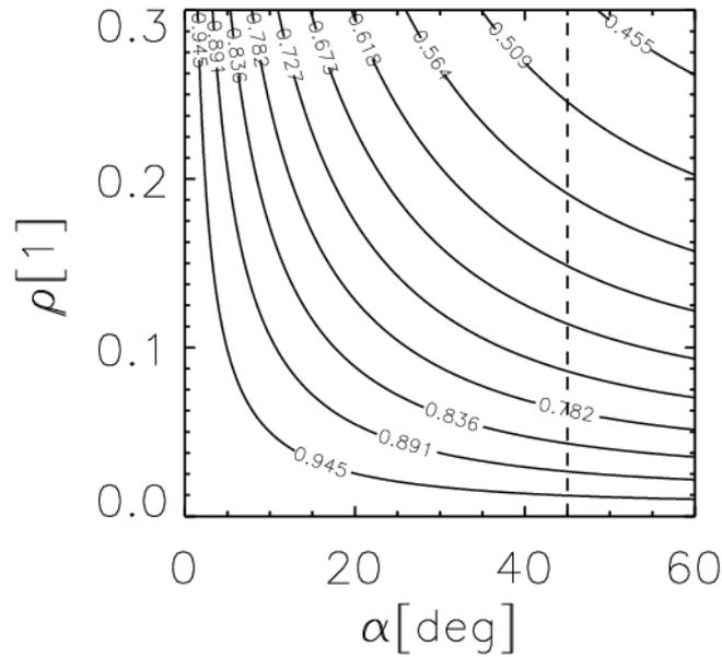
**Fig. 5 Equicontours of the power system mass efficiency propotional to the averaged modulation voltage over the maximum voltage to the power of 3/2.**
