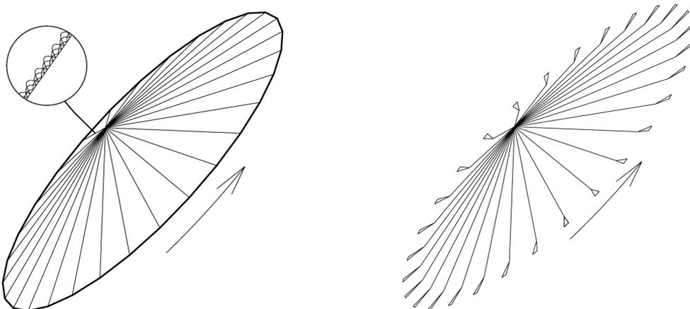
**Fig. 1 Electric sail designs use either auxiliary tethers and remote units (left) or Freely Guided Photonic Blades (right) for the sail flight time stability.**
