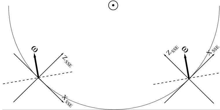
**Fig. 6 Slow rotation of the sail in the non-inertial SSE coordinate system while orbiting around the sun.**
